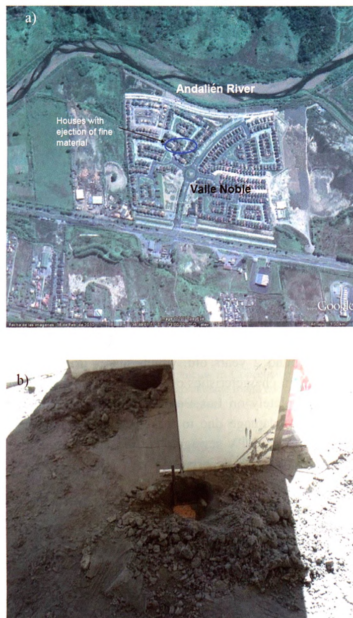
Figure 6: Valle Noble a) location of affected houses and b) large amount of fine material ejected inside a house up to 10cm thickness
