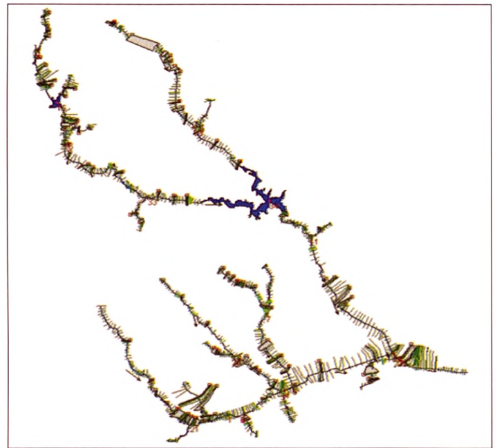
Figure 4. HEC-RAS Geometry Schematic for Cameron Run.
