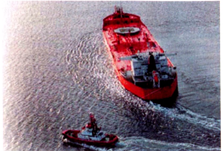
Figure 4: Tanker being steered using a tethered stern tug
