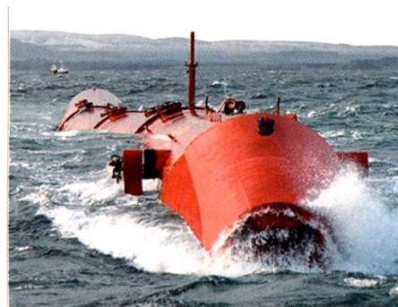
Figure 9: Pelamis P750 device [9]
